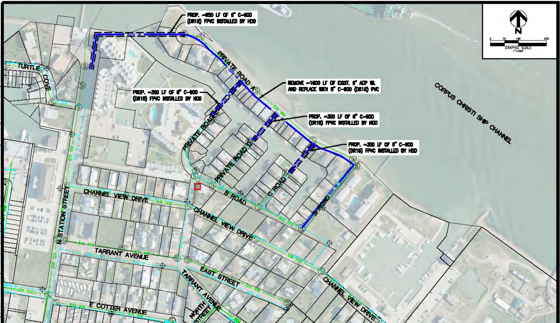
FIGURE VI-2 FIRE FLOW IMPROVEMENTS PRIVATE ROAD A WATERLINE NUECES COUNTY WATER CONTROL AND IMPROVEMENT DISTRICT #4
