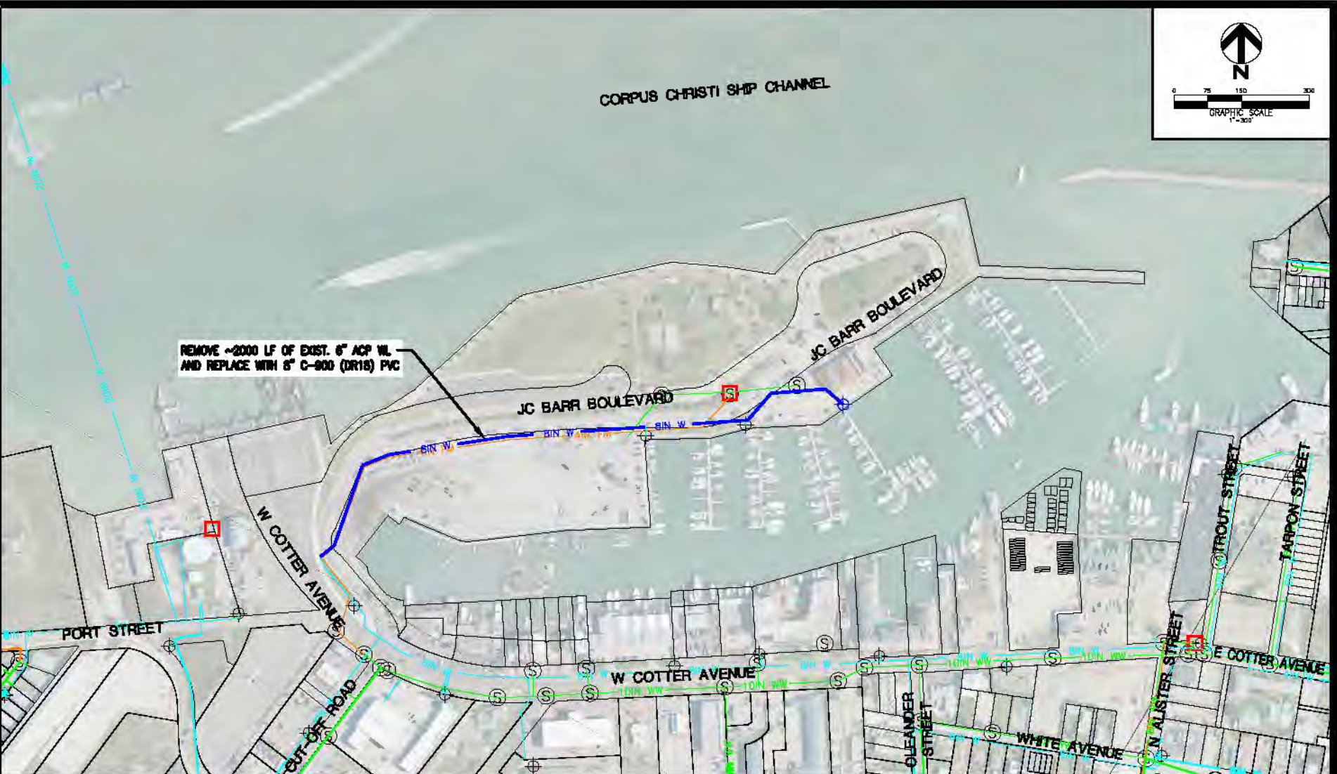
FIGURE VI-1 FIRE FLOW IMPROVEMENTS MARINA 6" WATERLINE TO 8" WATERLINE NUECES COUNTY WATER CONTROL AND IMPROVEMENT DISTRICT #4
